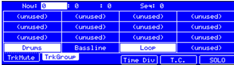
The Track Mute display of the MPC hardware
